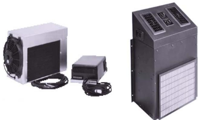
**The Telecom Self –Contained DC 17000T** controlled by a thermostat that senses the internal enclosure temperature. When cooling is desired, the compressor, evaporator blower and condenser fan turn on. Cool air is discharged from the DC Comfort T Series into the enclosure.
